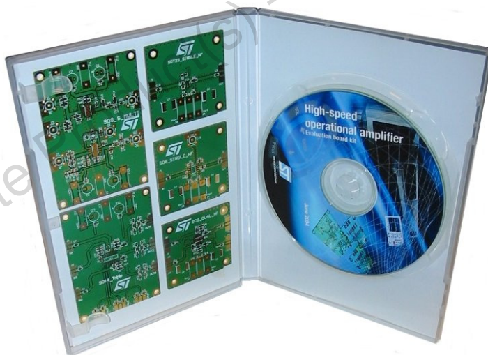
Figure 25: Evaluation kit for high-speed op-amps
