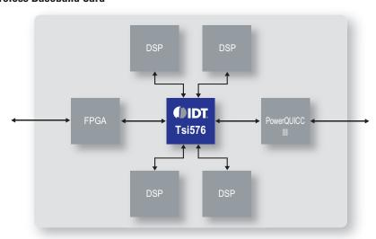
In video infrastructure cards, equipment vendors must maximize the number of DSPs per card to manage compression and decompression algorithms. These DSPs are controlled by a local processor and all these components are linked together by a low power, small form factor, low latency, multicast enabled Tsi576.
