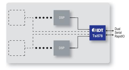
The Tsi578 provides traffic aggregation through packet prioritization when it is used with RapidIOenabled I/O devices. When it is in a system with multiple RapidIO-enabled processors it provides high performance peer-to-peer communication through its non-blocking switch fabric.
