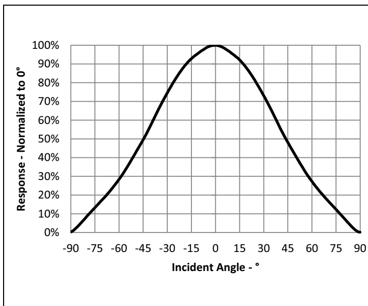
Figure 13: Ch0 Response to White LED (CCT = 4000K) vs. Incident Angle
