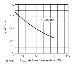
Fig. 7 - Rel. Radiant Intensity/Power vs. Ambient Temperature
