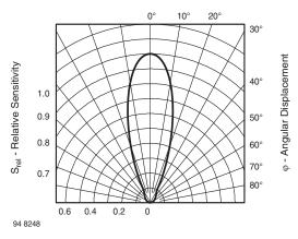
Fig. 9 - Relative Radiant Intensity vs. Angular Displacement
