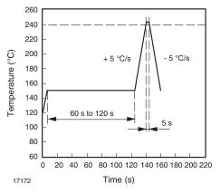
Fig. 10 - Lead Tin (SnPb) Reflow Solder Profile
