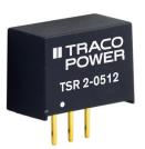
The new TSR 2 series step-down switching regulators are drop-in replacement for inefficient LMxx linear regulators. A high efficiency up to 96 % allows full load operation up to  $+67^{\circ}$ C ambient temperature without the need of any heat-sink or forced cooling.
