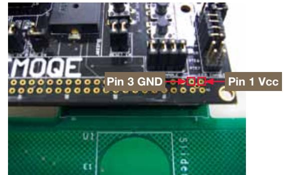
3. Connect pins 1 and 3 from the DEMO board to pins 1 and 3 respectively and insert the whole connector.
