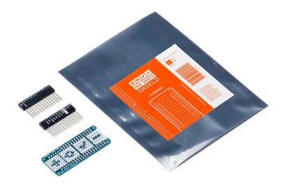
The MKR Proto Shield is a prototyping shield designed for your MKR board. This shield easily plugs onto your MKR using its provided female/male headers, and offers a duplicate breakout for each pin on the board along with many solderable through-holes on a standard 0.1" grid (2.54mm).
