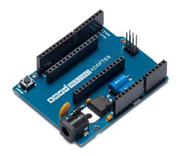
The MKR2UNO Adapter allows you to easily turn your Arduino UNO form factor project into an MKR-based one! Take your creations to the next level with a powerful IoT board featuring an integrated LiPo battery charger.
