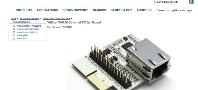
WIZnet's W5200 Ethernet PICtail™ (Plus) board provides 10/100Mbps, half/full duplex Ethernet connectivity by onboard WIZnet W5200 Ethernet controller, which has a hardwired TCP/IP processing engine.
