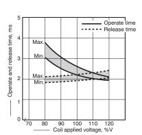
6-(2). Operate and release time (without diode) Tested sample: TX2-5V, 10 pcs.
