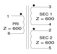
BOTH SECONDARIES MUST BE LOADED FOR IMPEDANCE SPECIFICATIONS TO BE ACCURATE.
