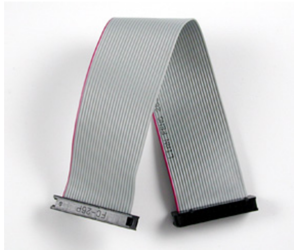
Figure 3-15: ColdFire Ribbon Cable (for asynchronous ColdFire targets, included with Cyclone)
