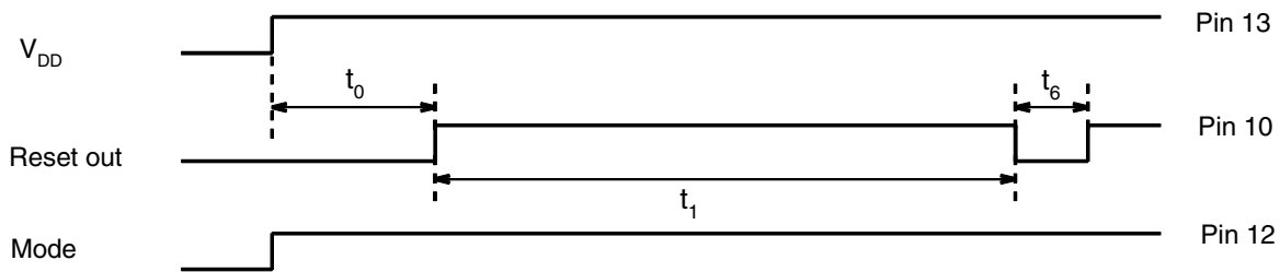
Figure 4-2. Power-up Reset and Mode Switchover
