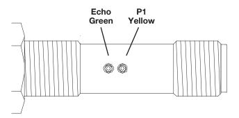
The Echo LED is ON when an echo is received (alignment
