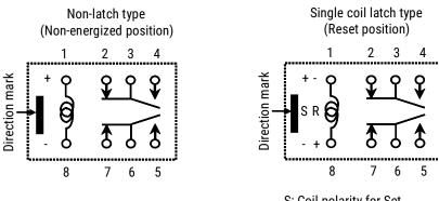
S: Coil polarity for Set R: Coil polarity for Reset
