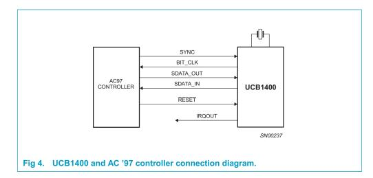
The UCB1400 implements an AC '97 Revision 2.1 interface. Refer to the *Audio Codec '97 Component Specification Revision 2.1* from Intel.
