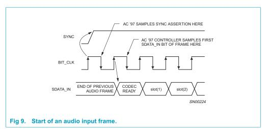
SDATA\_IN's composite stream is MSB justified (MSB first) with all non-valid bit positions (for assigned and/or unassigned time slots) stuffed with 0s by the UCB1400. SDATA\_IN data is sampled on the falling edges of BIT\_CLK.
