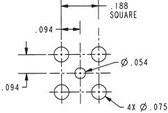
RECOMMENDED MTG HOLE PATTERN SCALE 3/I
