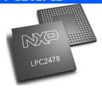
The NXP LPC2478 ARM7TDMI-S based microcontroller runs the open source uEZ® + FreeRTOS software platform. The LPC2478 has 512KB of internal Flash memory, 96KB of internal SRAM, a 10/100 Ethernet Media Access Controller (MAC), a USB full speed device/host/OTG controller, four UARTs, two CAN channels and a collection of serial communications interfaces. The uEZGUI board also includes 8MB of external SDRAM and 8MB of external NOR Flash
