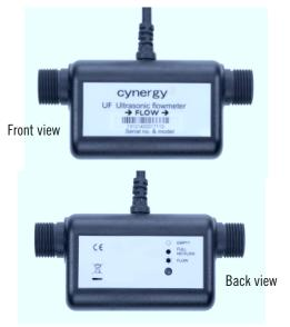
This innovative design provides a high accuracy, non-invasive, flow measurement device at a fraction of the cost of other current non-invasive systems. The unique measurement technique automatically compensates for viscosity and temperature variations. The measurement of flow is by ultrasonic transit time in-line cell.
