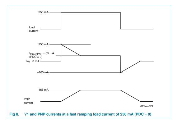
For short-circuit protection, a resistor needs to be connected between pins V1 and VEXCC to allow the current to be monitored. This resistor limits the current delivered by the external transistor. If the voltage difference between pins VEXCC and V1 reaches  $V_{th(act)|llim}$ , the PNP current limiting activation threshold voltage, the transistor current will not increase further.
