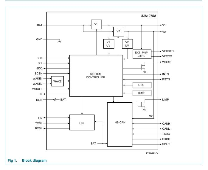
High-speed CAN/LIN core system basis chip
