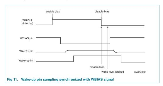
The sampling of the wake-up pins can be synchronized with the WBIAS signal by setting bits WSE1 and WSE2 in the Int\_Control register to 1 (if WSEx = 0, wake-up pins are sampled continuously). The sampling will be performed on the rising edge of WBIAS (see Figure 11). The sampling time, 16 ms or 64 ms, is selected via the Wake Bias Control bit (WBC) in the Mode\_Control register.
