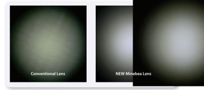
Our newly developed lens provides higher quality color uniformity and a significantly smaller structure when compared with conventional lenses.
