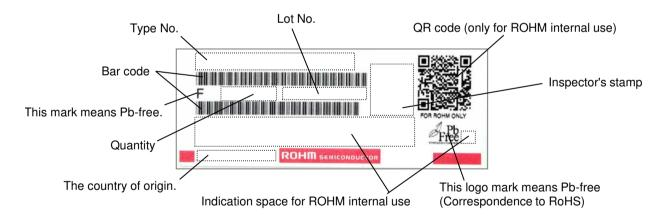
9. Type Product code of taping shall be composed as indicated below.
