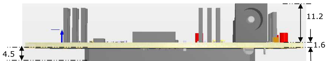
Figure 2-6 UMFT600A/UMFT601A Dimensions (Side view)
