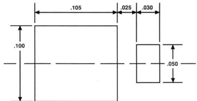
Figure 1. Suggested Mounting Pad Dimensions
