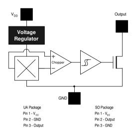
**Note:** This is a static-sensitive device; please observe ESD precautions. Reverse  $V_{DD}$  protection is not included. For reverse voltage protection, a  $100 \Omega$  resistor in series with  $V_{DD}$  is recommended.
