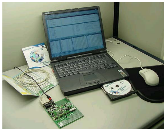
Figure 1. The ADuC8xx QuickStart Development System
