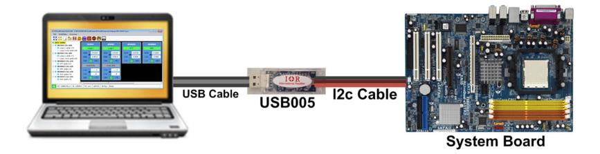
Provide interface between IR PowIRCenter GUI and the IR controllers
