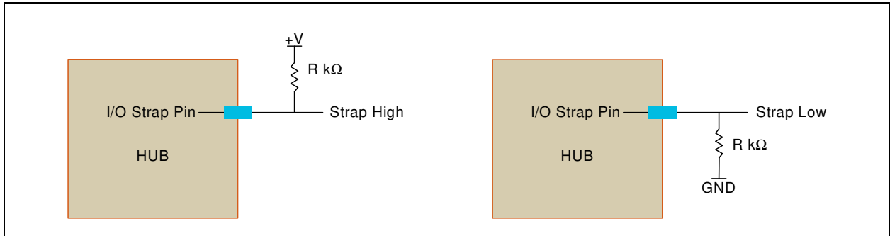
FIGURE 2-2: NON-REMOVABLE PIN STRAP EXAMPLE
