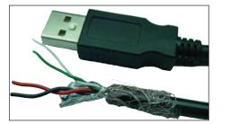
General Construction: this is a USB-2.0 cable containing one 28 AWG 90 $\Omega$  characteristic impedance data pair, two 24 AWG power conductors, overall SFTP shields (SFTP = double shielding, Braid and foild), jacketed in black UV resistant Polyurethane HFFR\*. Designed for fixed or portable applications in industrial and harsh environments.\*HFFR: Halogen Free Flame Retardant.
