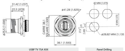
Jam nut receptacle Hexagonal Nut mounting: Shell type 7
