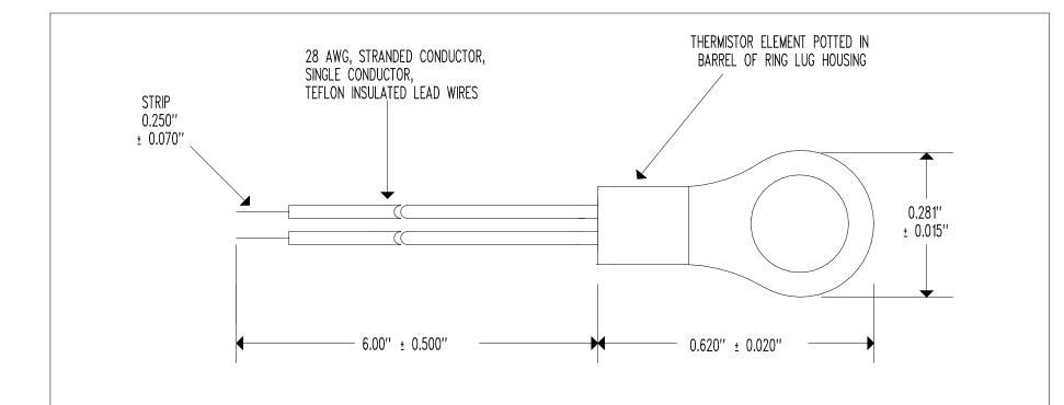
RESISTANCE @ +25'C =  $10,000 \Omega \pm 1\%$ RESISTANCE/TEMPERATURE CURVE = "J" TEMPERATURE COEFFICIENT @ +25'C = -4.4%/'C NOMINAL BETA " $\beta$ " (0 TO +50'C) = 3,892'K NOMINAL MAXIMUM TEMPERATURE RATING = +150'C
