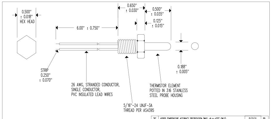
RESISTANCE @  $+25^{\circ}C$  = 10,000  $\Omega$  NOMINAL ACCURACY (0 TO  $+60^{\circ}C$ ) =  $\pm$  1.0°C RESISTANCE/TEMPERATURE CURVE = "E1" BETA " $\beta$ " (+25 TO  $+85^{\circ}C$ ) = 3,435°K NOMINAL MAXIMUM TEMPERATURE RATING =  $+105^{\circ}C$
