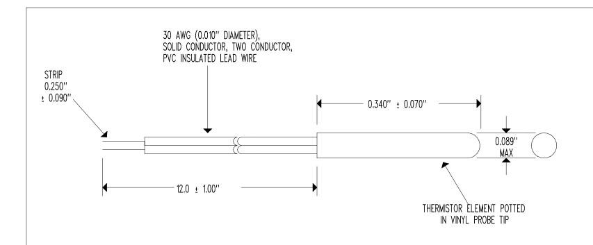
RESISTANCE @  $+25^{\circ}C$  = 10,000  $\Omega$  ± 1% RESISTANCE/TEMPERATURE CURVE = "J" TEMPERATURE COEFFICIENT @  $+25^{\circ}C$  = -4.4%/°C NOMINAL BETA " $\beta$ " (0 TO  $+50^{\circ}C$ ) = 3,892°K NOMINAL MAXIMUM TEMPERATURE RATING =  $+80^{\circ}C$
