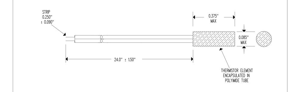
RESISTANCE @  $+25^{\circ}C$  = 10,000  $\Omega$  NOMINAL ACCURACY (0 TO  $+50^{\circ}C$ ) =  $\pm$  0.10°C RESISTANCE/TEMPERATURE CURVE = "J" BETA " $\beta$ " (0 TO  $+50^{\circ}C$ ) = 3,892°K NOMINAL TEMPERATURE COEFFICIENT @  $+25^{\circ}C$  = -4.4%/°C NOMINAL MAXIMUM TEMPERATURE RATING =  $+105^{\circ}C$
