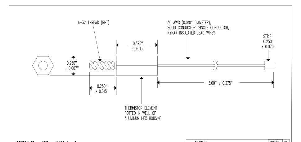
RESISTANCE @  $+25^{\circ}C = 10,000 \Omega \pm 5\%$ RESISTANCE/TEMPERATURE CURVE = "J" BETA " $\beta$ " (0 TO  $+50^{\circ}C$ ) = 3,892'K NOMINAL TEMPERATURE COEFFICIENT @  $+25^{\circ}C = -4.4\%$ /'C NOMINAL MAXIMUM TEMPERATURE RATING =  $+125^{\circ}C$
