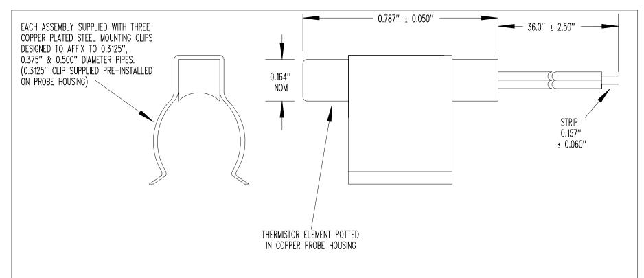
RESISTANCE @  $+25^{\circ}$ C = 10,000  $\Omega$  ± 1% RESISTANCE/TEMPERATURE CURVE = "J" TEMPERATURE COEFFICIENT @  $+25^{\circ}$ C = -4.4%/°C NOMINAL BETA " $\beta$ " (0 TO  $+50^{\circ}$ C) = 3,892°K NOMINAL MAXIMUM TEMPERATURE RATING =  $+105^{\circ}$ C
