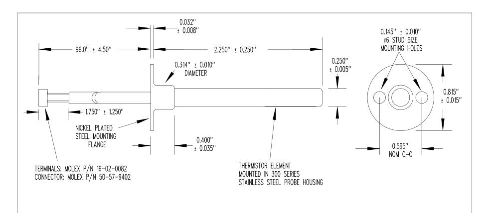
RESISTANCE @  $+25^{\circ}C = 100,000 \Omega \pm 2\%$ RESISTANCE/TEMPERATURE CURVE = "J" BETA " $\beta$ " (0 TO  $+50^{\circ}C$ ) = 3,892°K NOMINAL TEMPERATURE COEFFICIENT @  $+25^{\circ}C = -4.4\%$ °C NOMINAL MAXIMUM TEMPERATURE RATING =  $+300^{\circ}C$
