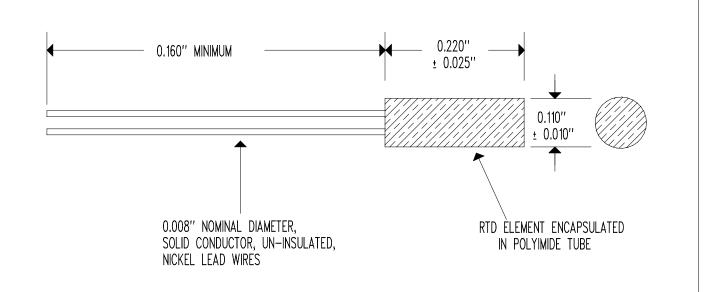
RESISTANCE @ 0°C =  $500 \Omega \pm 0.12\%$ ACCURACY @ 0°C =  $\pm 0.30$ °C DIN 43760 ACCURACY CLASS = "B" TCR = 3.850ppm/°C MAXIMUM TEMPERATURE RATING = +150°C
