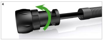
Screw the fitting onto the plug thread. Use a product such as Loctite to ensure adequate sealing between the plug and the fitting.
