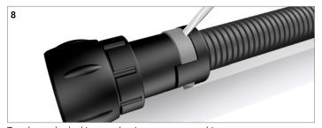
To release the locking mechanism, use a screwdriver.
