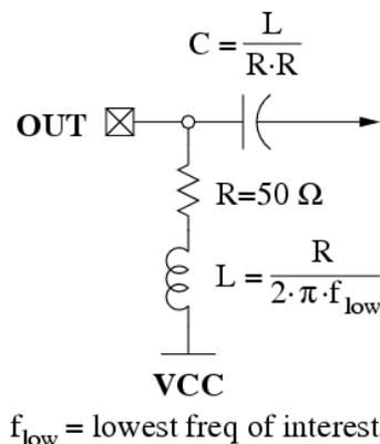
In addition to the maximum input signal levels, single-ended operation imposes additional restrictions: the average DC value of the waveform at IC should be equal to Vcc for single-ended operation. In practice, this is easily achieved with a single capacitor on the input acting as a DC block. The value of the capacitor should be large enough to pass the lowest frequencies of interest.
