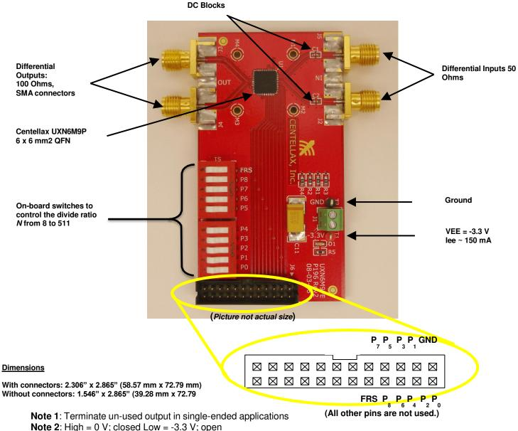
**Note 3**: When using the parallel programming interface control, <u>all on-board switches must be kept in the</u> 'open' position. 'Open' corresponds to logic 'Low' or 0. Refer to the datasheet for logic level specs. **Note 4**: Set FRS=High for Fin > 6 GHz
