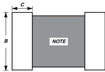
Note: Avoid metal runs in this area, parts are not recommended for use in applications using Silver (Ag) epoxy paste.
