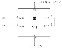
Measuring a current referenced to a floating supply, i.e. the current being measured and the meter's power supply are isolated from each other. Check Link L1 is closed.
