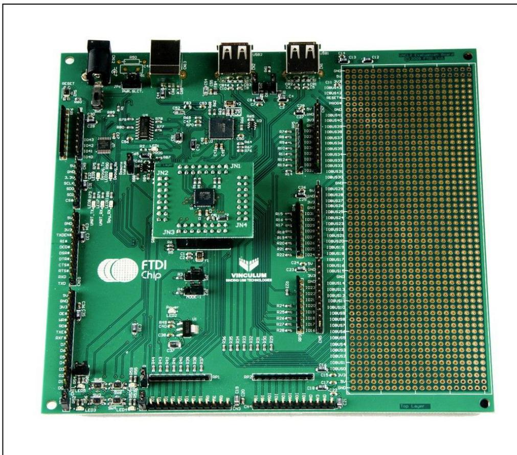
Figure 4.1 V2-EVAL Board with VNC2 Daughterboard Installed
