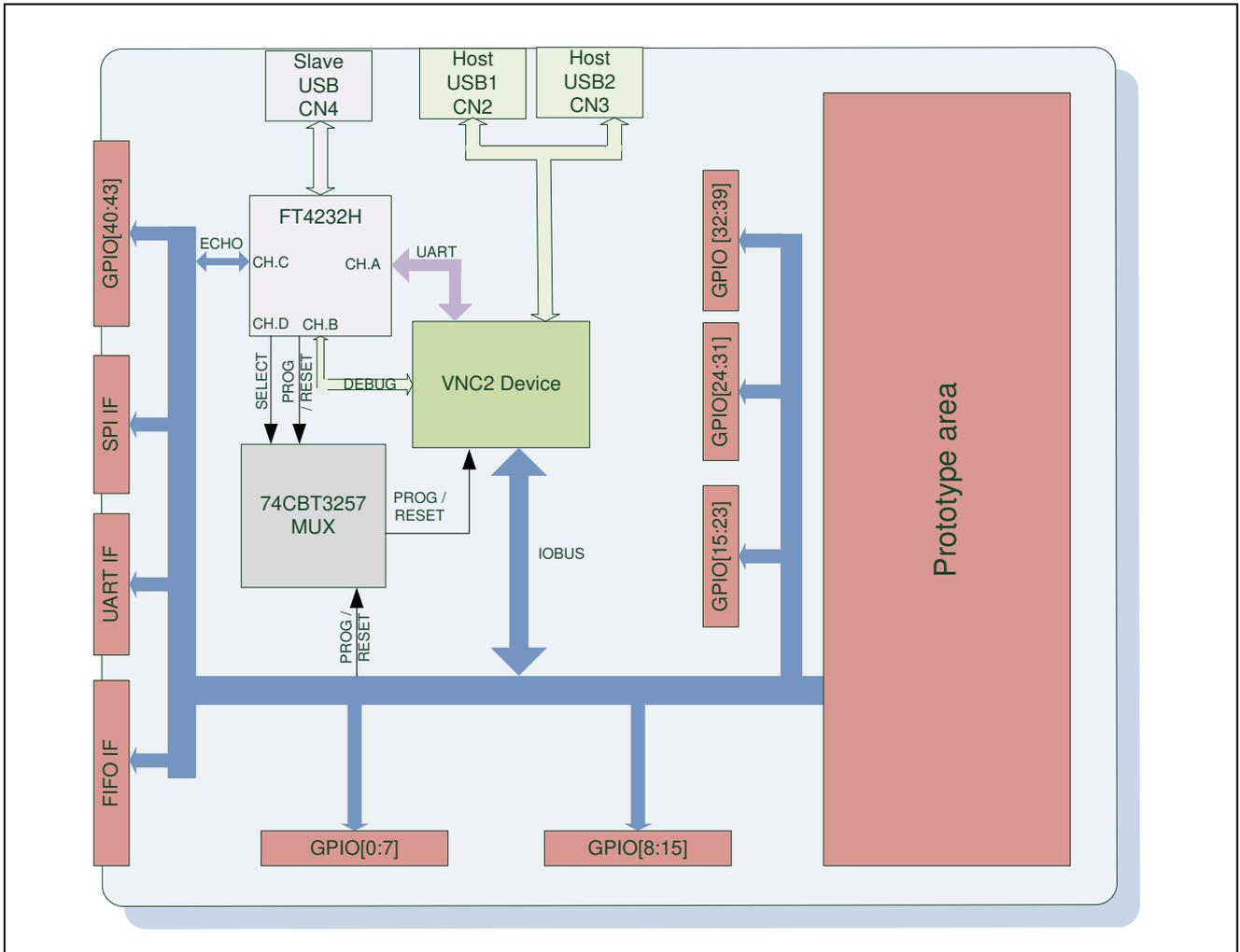
Figure 3.2 V2-EVAL Board Block Diagram
