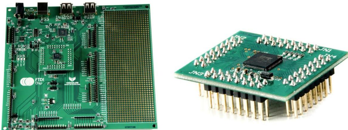
Figure 1.1 - V2-EVAL Motherboard(left) with Daughterboard Module(right)
