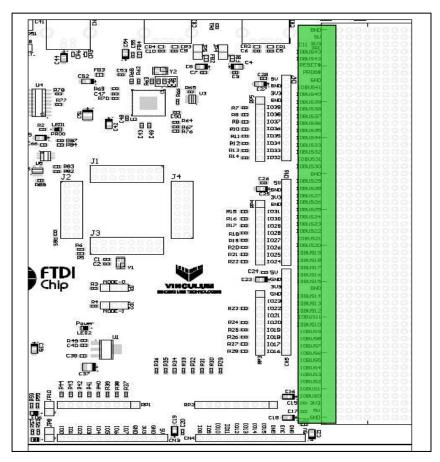
Figure 5.11 Prototyping area P1
