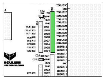
Figure 5.5 GPIO[24:31] Connector CN6
