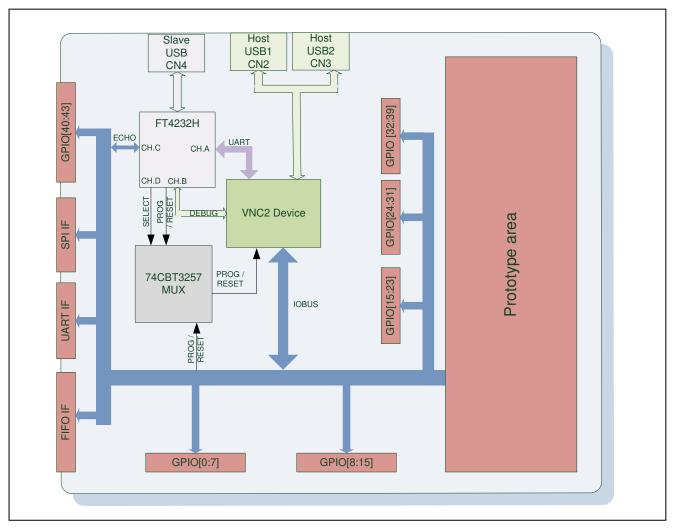
Figure 3.2 V2-EVAL Board Block Diagram
