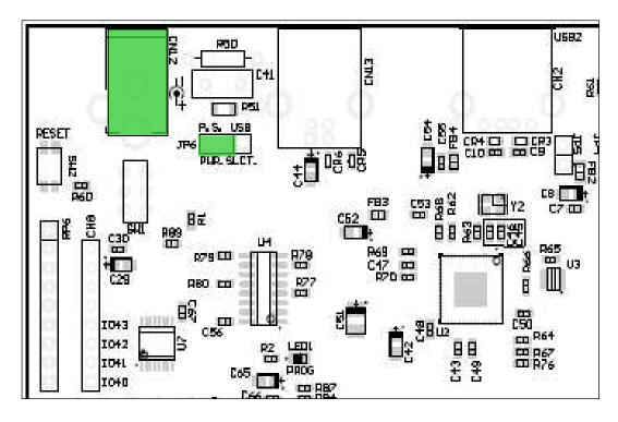
Figure 4.2 Power connector with Jumper JP6
