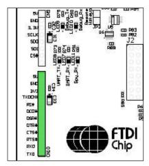
Figure 5.9 UART Connector CN10
