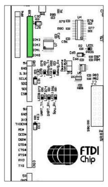
Figure 5.7 GPIO[32:39] Connector CN8
