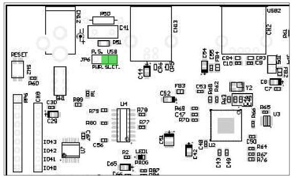
Figure 5.1 Power Select Jumper Configuration for USB Power
