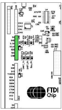
Figure 5.8 SPI Connector CN9
