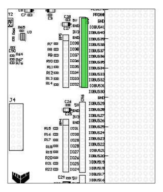
Figure 5.6 GPIO[32:39] Connector CN7
