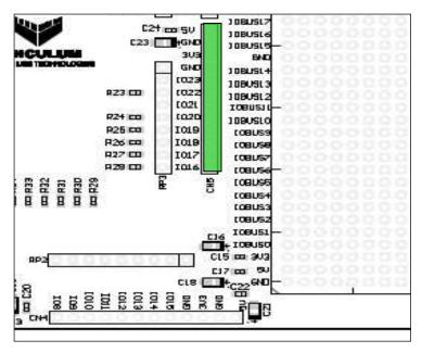
Figure 5.4 GPIO[16:23] Connector CN5
