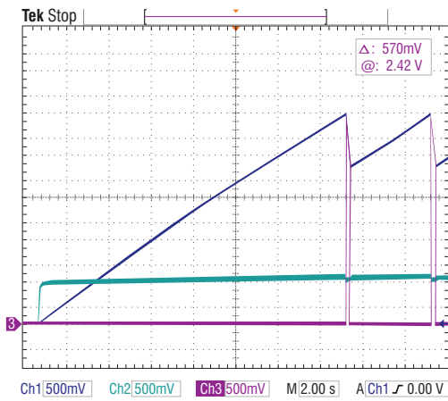
Figure 5: Rectified input (aqua), V_{CAP} (navy) and switched output (violet) from initial start-up to stable output, 10K resistive load.
