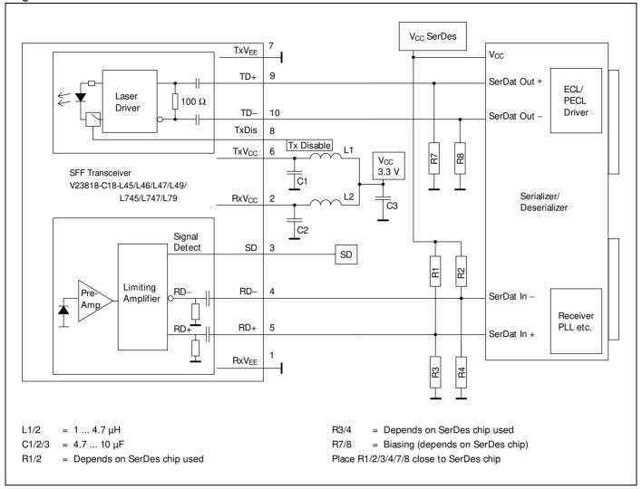
Values of R1/2/3/4 may vary as long as proper 50  $\Omega$  termination to V<sub>FF</sub> or 100  $\Omega$  differential is provided. The power supply filter-
