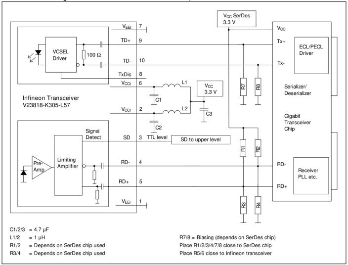
Values of R1/2/3/4 may vary as long as proper 50  $\Omega$  termination to V<sub>EE</sub> or 100  $\Omega$  differential is provided. The power supply filter-
